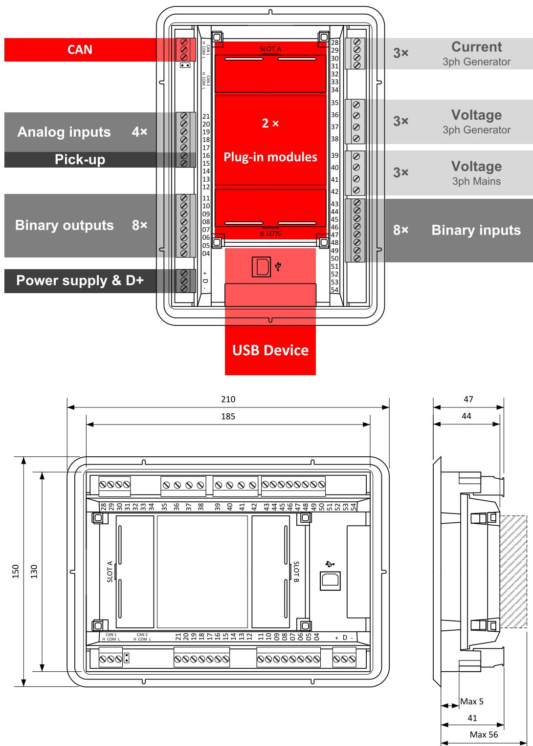
**Note:** The final depth of the controller depends on the selected plug-in module – it can vary between 41 mm and 56 mm. Mind also the size of connectors and cables (e.g. in case of RS232 connector, add about 60 mm more for standard RS232 connector and cable).
