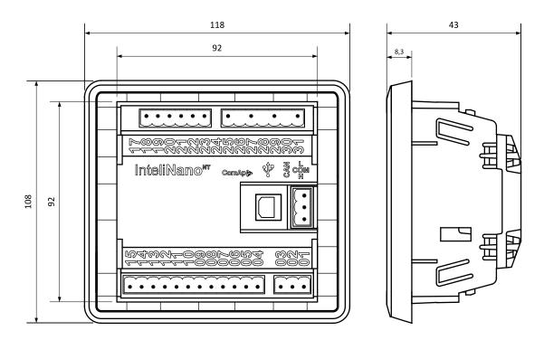
**Note:** The controller is to be mounted into panel doors as a standalone unit using provided fixing clips. The requested cut-out size is  $94 \times 94$  mm. Use the screw holders delivered with the controller to fix the controller into the door.
